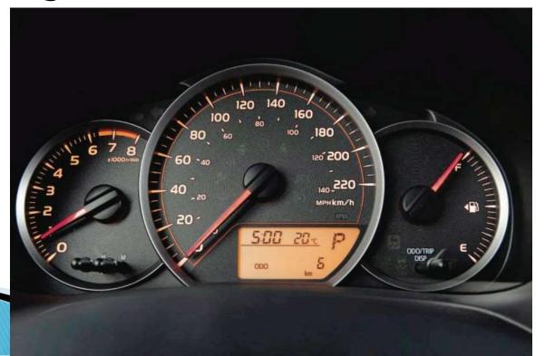
Odometer: Odometer is a device on the dashboard of the vehicle which gives the measure of the distance covered by the vehicle.
