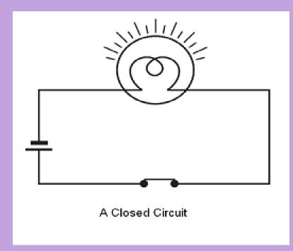
• When the key is switched on or closed, the circuit is said to be closed or complete. As the circuit is complete, the bulb starts glowing. What happens when the filament of a bulb breaks? When the filament of a bulb breaks, the circuit becomes incomplete. Hence, the bulb does not glow.
