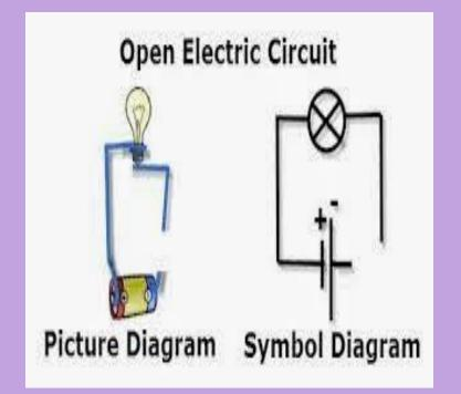
• When the key is in switch off condition or open the circuit is said to have open electric circuit. The circuit is incomplete so the bulb attached to it does not glow.
