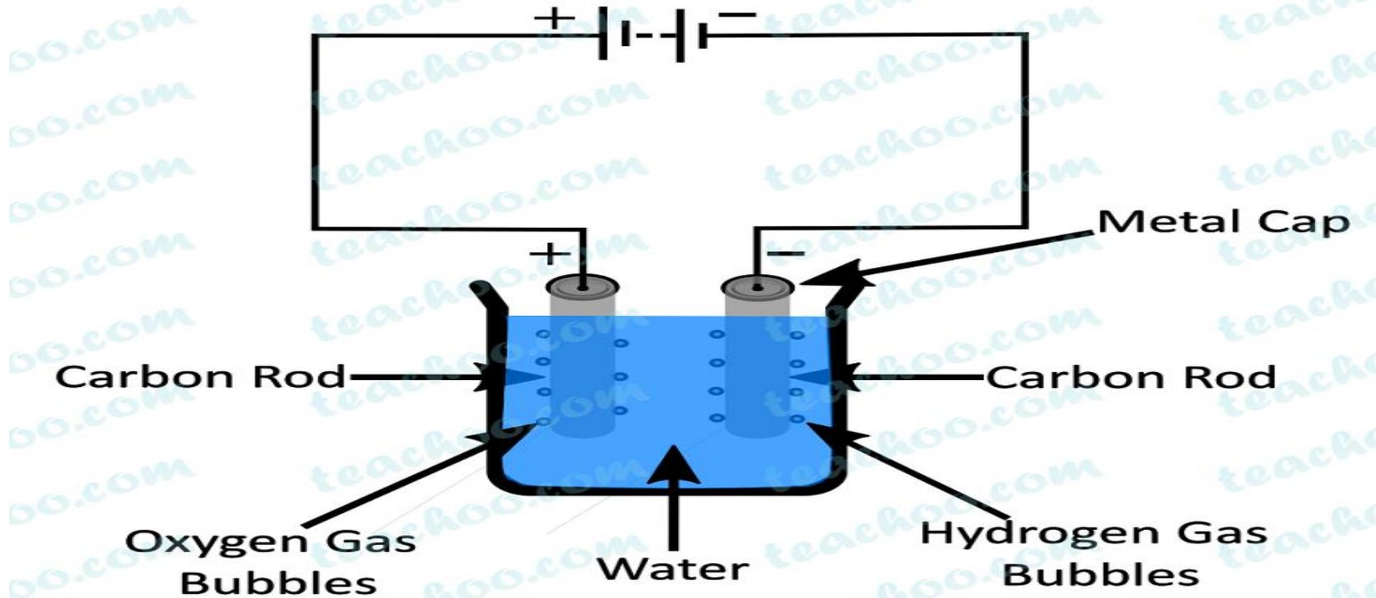
Oxygen bubbles formed on the electrode connected to the positive terminal of the battery and hydrogen bubbles formed on the electrode connected to the negative terminal of the battery.
