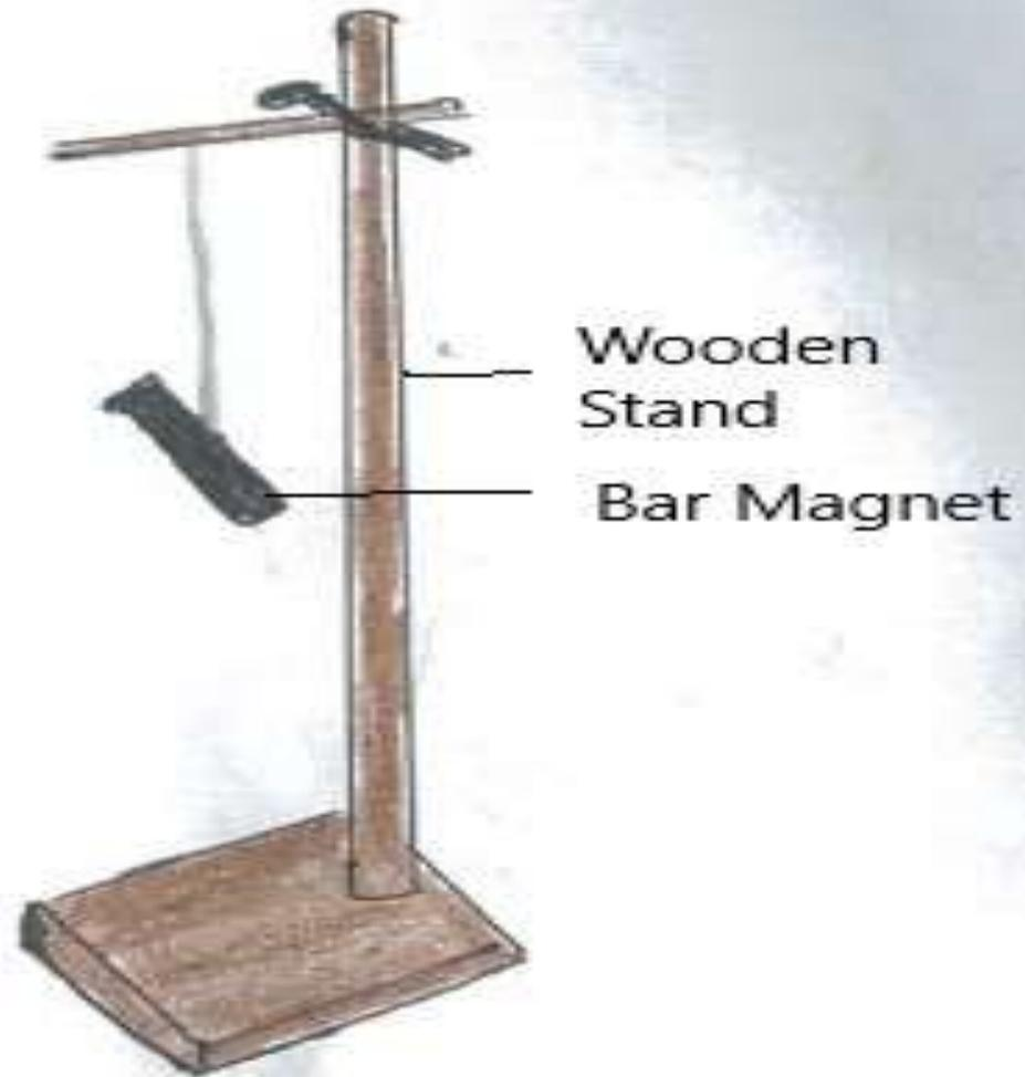
A freely suspended bar Magnet always comes to rest in the same direction
