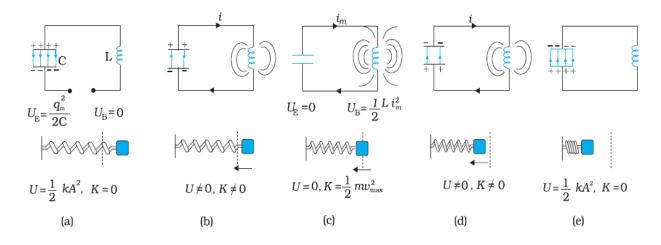
(a) At the initial stage, when the switch is opened, the energy stored in the capacitor is maximum. It is stored in the form of 'electrostatic potential energy ( $U_E$ ).
