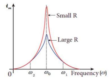
The maximum current at series resonance is limited by the resistance (R) of the circuit.
