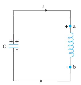
Let a capacitor be charged  $q_m$  (at t = 0) and connected to an inductor as shown in the above figure. The moment the circuit is completed, the charge on the capacitor starts decreasing, giving rise to current in the circuit. Let q and i be the charge and current in the circuit at time t. Since  $\frac{di}{dt}$  is positive, the induced emf in L will have polarity as shown, i.e.,  $v_b < v_b$ . According to Kirchhoff's loop rule,
